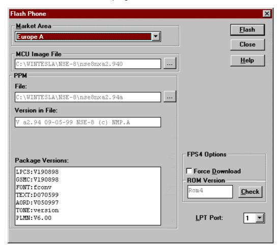
Flashing the phone supports both the FPS4 flash prommer setup and the FLS–X device. The device used is selected in the menu **Configure** | **FLS–1.** If **Use FLS–X** is checked then the FLS–X device is activated or else is the FPS4 prommer activated.
