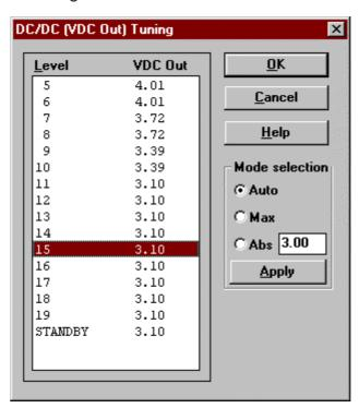
The DC/DC converter can be set to 3 different modes. When opening the DC/DC tuning dialog the currently used mode is shown.
